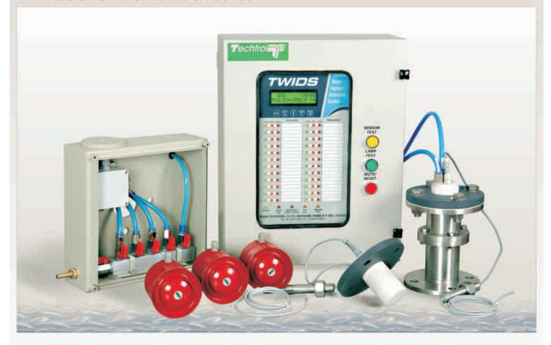
TWIDS consists of a control panel and a set of two water detectors in each hold. An audio / visual alarm is annunciated in case of water ingress in any hold / dry space. The control panel provides individual indication for status, fault & alarm for each cargo hold with distinct signals for pre & main alarm levels.
